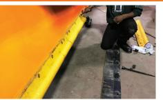
EASY TO INSTALL 3FT AND 4FT SECTIONS FOR PLOWS AND WINGS
